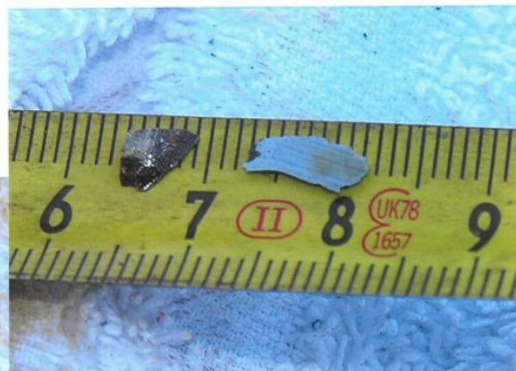
Particles found in the bottom of the gearbox with a magnet.
