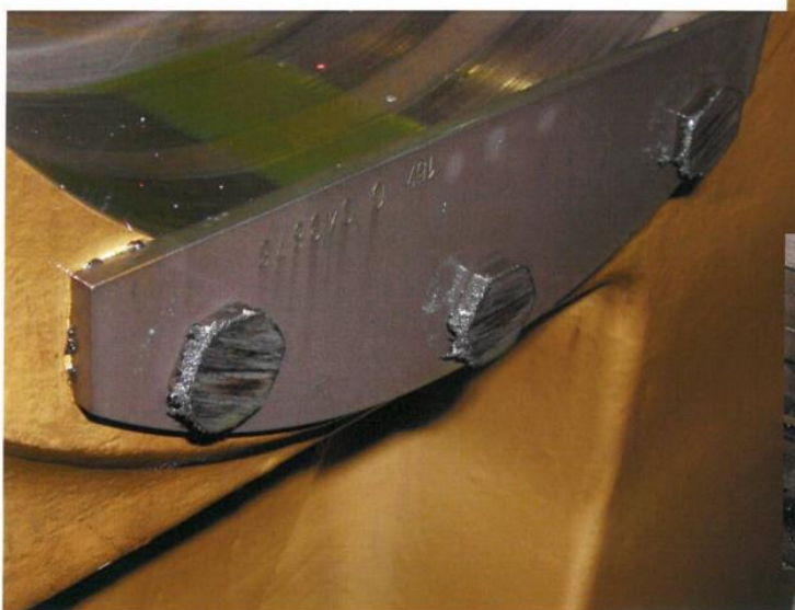
HS IMS wheel has worn 3 bolt heads ~10 mm.
