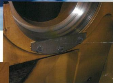
HS IMS wheel has worn 3 bolt heads ~10 mm.
