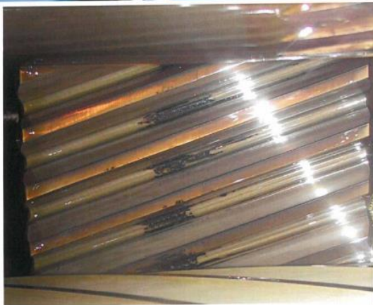
HS IMS pinion Stand still marks Indentation marks and scuffing from particles
