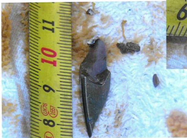
Particles found in the bottom of the gearbox with a magnet.
